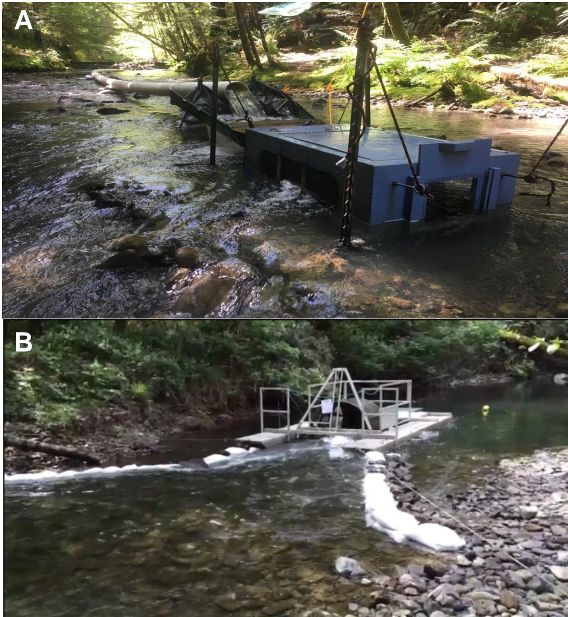
Figure 2. Photos showing the trapping methods, V-notch weir/pipe trap (A) and RST (B), used for outmigrant trapping in Little River, Humboldt County, California.
